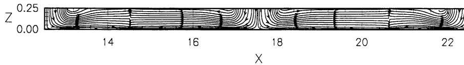
Fig. 8. Projection of flow lines on mid  $x-z$  plane for  $Re = 200$ ,  $A_z = 0.25$  and  $X_n = 5$ .
